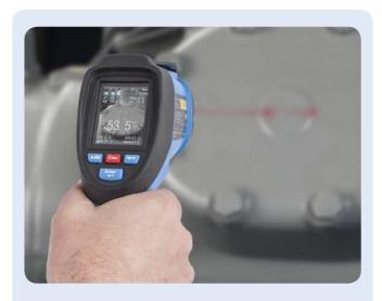
When used in non-contact mode, the thermometer senses the thermal energy radiated from an object with an infrared detector. When pointed at an object, the infrared detector collects energy, producing a signal that the microprocessor translates as a reading on the backlit display.
